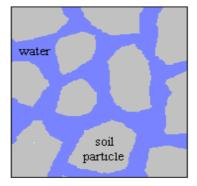
Figure 1b – Soil at field capacity Spaces between the soil particles filled with water and air
