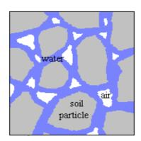
Figure 1c – Soil at wilting point Spaces mostly filled with air, with
